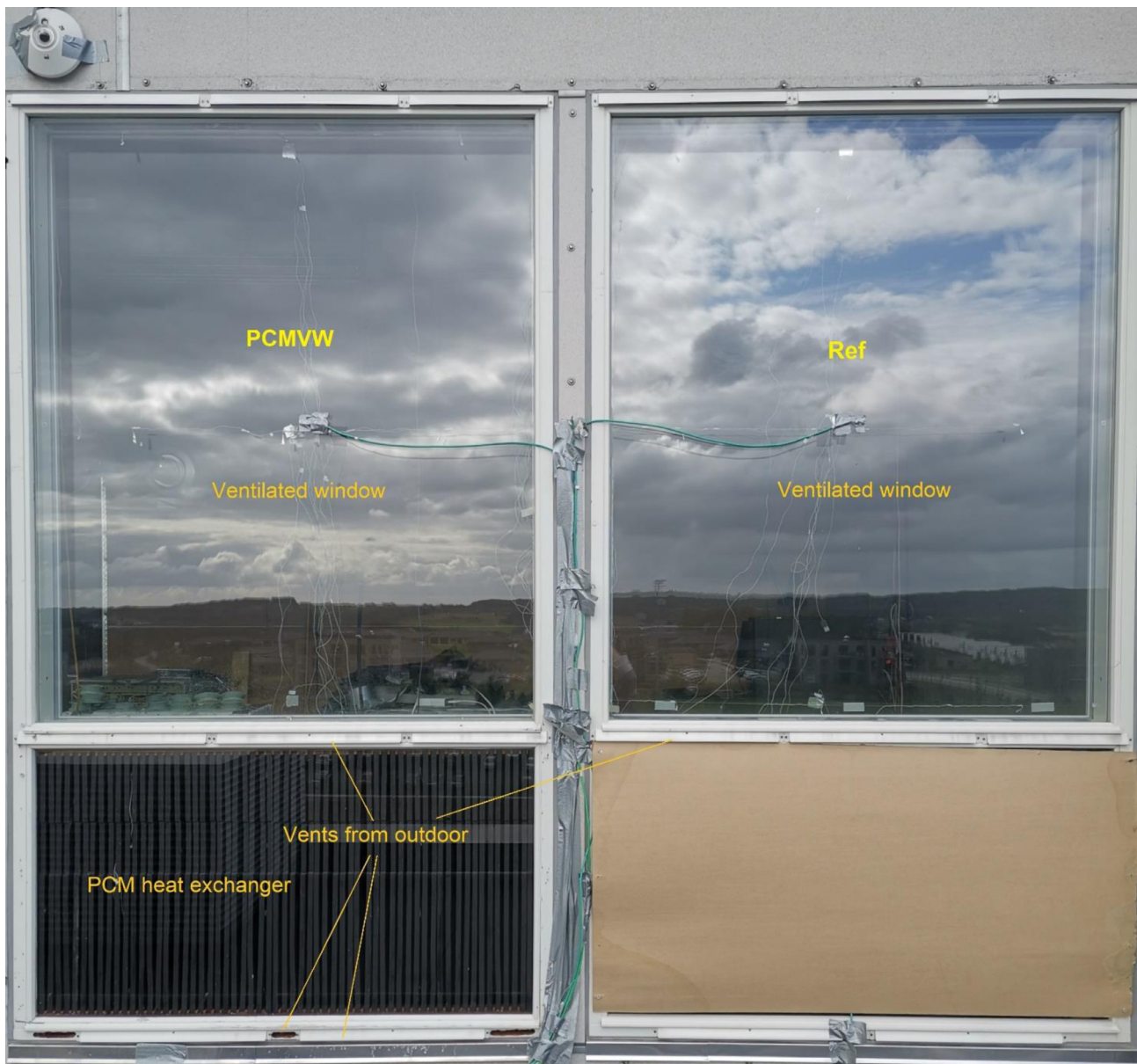
Fig. 1. Experimental setup. The PCMWW in the left and the Reference window in the right.
