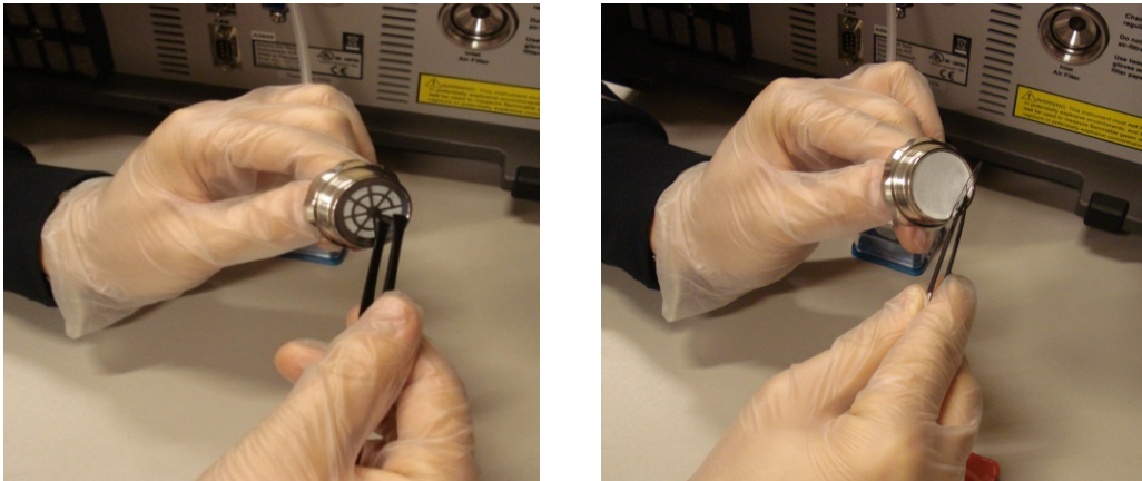
Figure 3. Lifting the metal ring by a tweezers.
