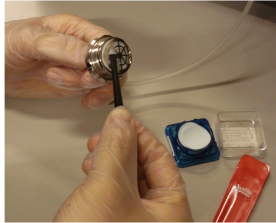
Figure 5. Placing a) new paper filter inside the internal filtration unit and b) the metal ring above new paper filter.
