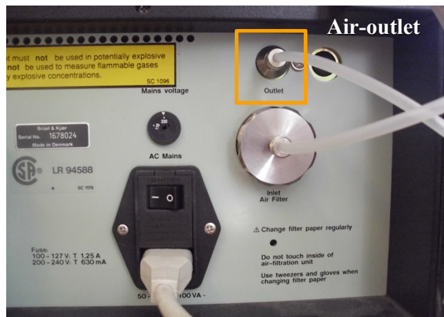
Figure 13. Monitor's back panel with highlighted air-outlet.
