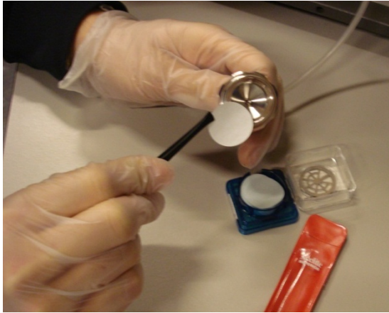
Figure 5. Placing a) new paper filter inside the internal filtration unit and b) the metal ring above new paper filter.
