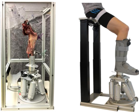
Fig. 1 - The in vitro version (left) of the 3D arthrometer used in the study and the in vivo version (right).
