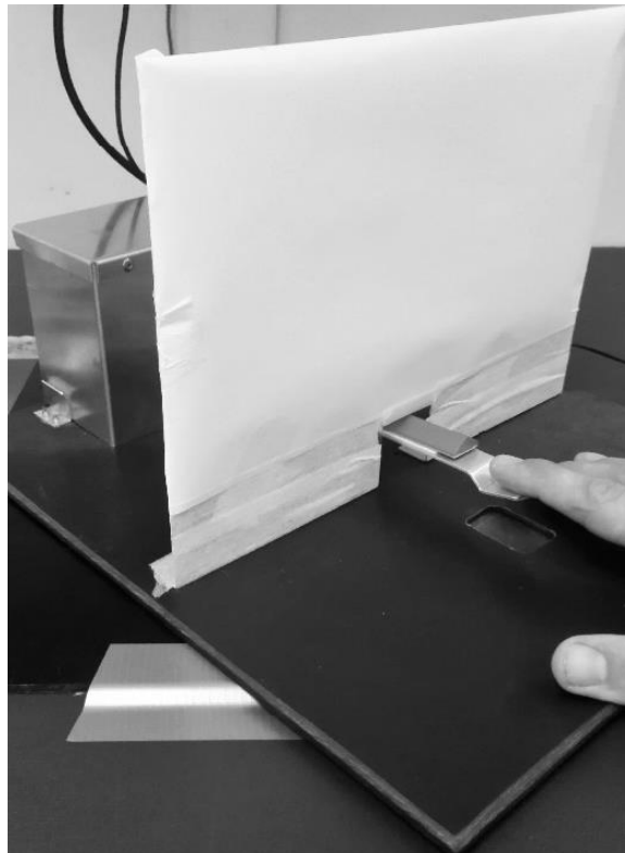
Figure 5. Illustration of the custom-built machine used to apply passive tapping in studies I-II. Adopted from study I (Emanuelson et al. 2018).
