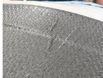
(d) Wrinkles developed from air pockets during debulking.
