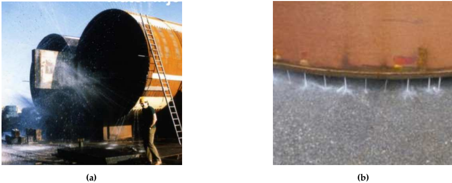
Fig. 1.10: (a) Nozzle system on bucket skirt tip used for Gullfaks C platform and (b) for OWT Trial Installation tests (Tjelta, 2014)
