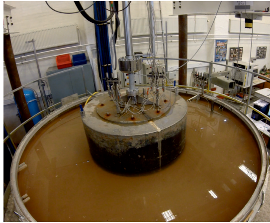
Fig. C.1: Laboratory installation test of a bucket model
