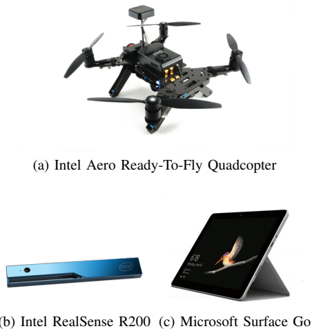
Fig. 1. Hardware setup used for the proposed framework
