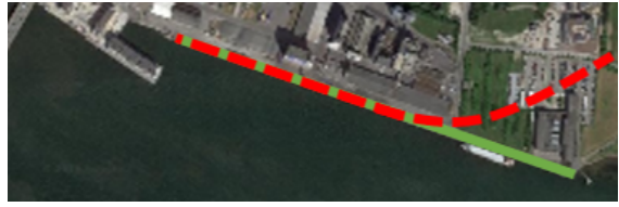
Figure 10: An illustration of a problem with the position estimation when panning to the right. The dotted red line is the position given by the estimator and the green line is the actual position of the waterfront.
