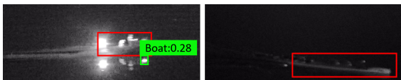
Figure 6: Output of retrained YOLOv3 on the optical image taken during the nights.
