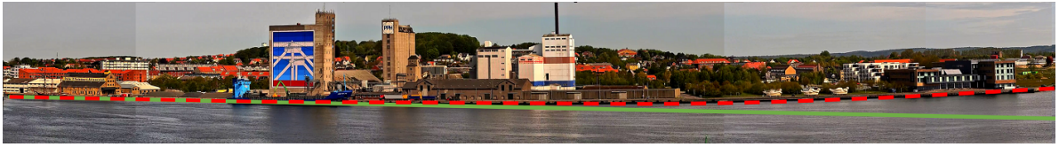
Figure 11: A panoramic image created of the waterfront. The dotted red line showing the waterfront as seen by the camera and the green line indicating the expected shape of the waterfront provided no panoramic distortion.
