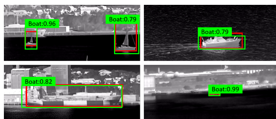
Figure 5: Output of retrained YOLOv3 on thermal images
