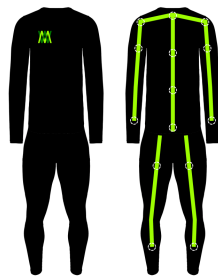
Figure 9: The Weight-Mate suit from (a) front and (b) back. The dotted circles indicate IMU locations.
