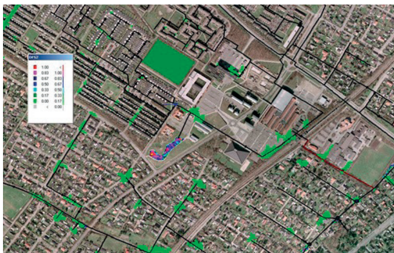
Figure 11. Simulated flooding for climate scenario A2 for the same rain as in Figure 10. The football field is used as flood storage (Paludan et al., 2010)
