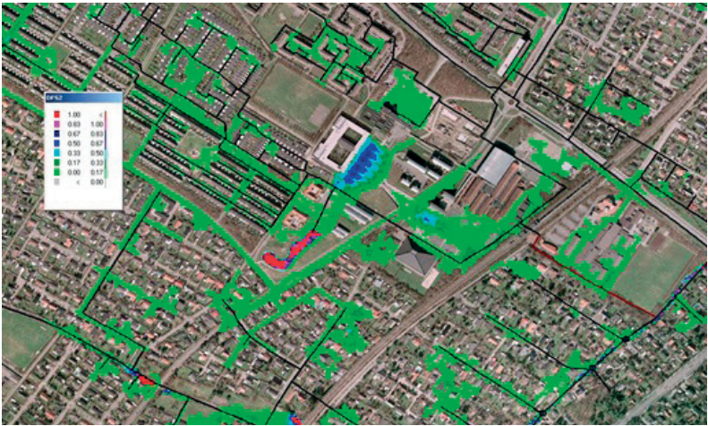
Figure 10. Simulated flooding for climate scenario A2 for rain with a 10-year return period in 2100 (Paludan et al., 2010)
