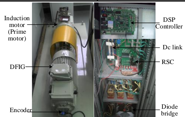
Fig. 6. Experimental set up of DFIG-DC system.
