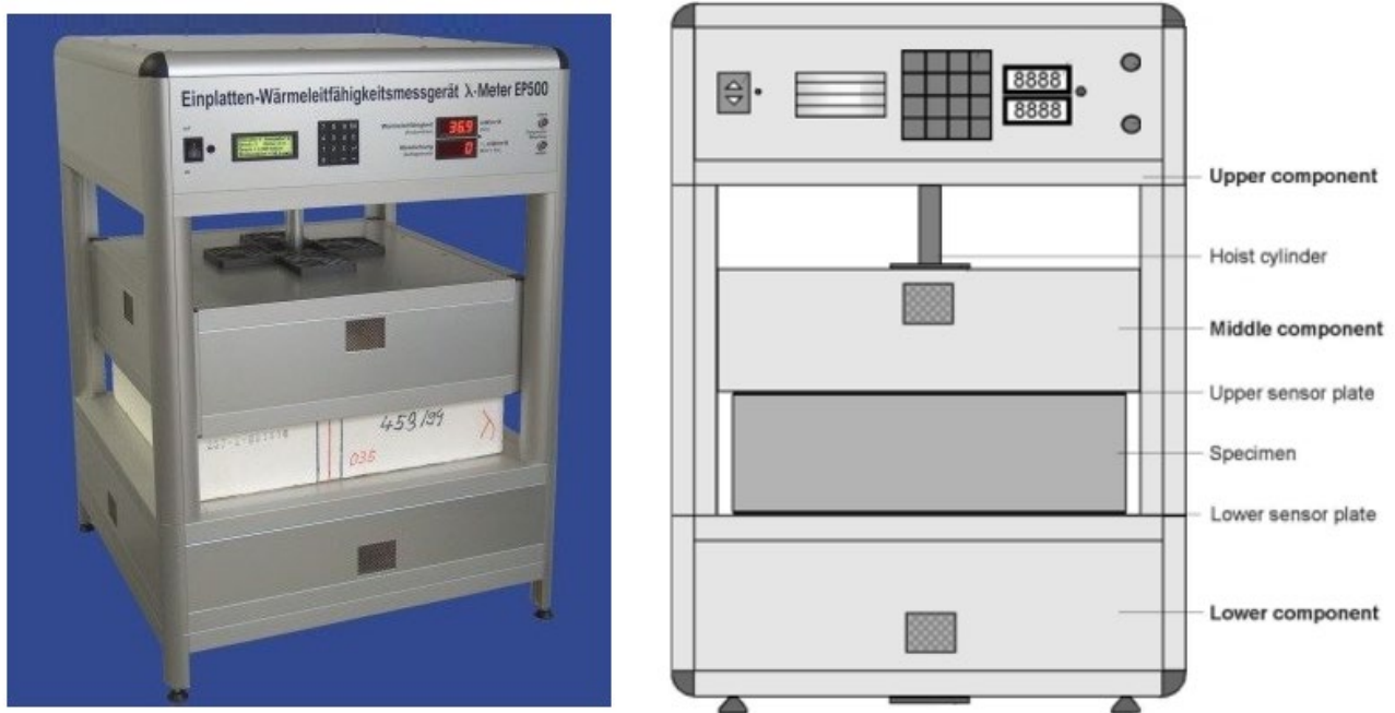
Figure 6: The Guarded Hot Plate apparatus EP500 from Lambda-Messtechnik GmbH Dresden [1].
