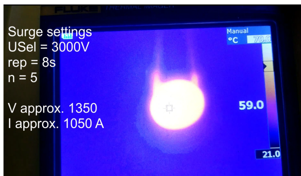
Fig. 9. Experimental recording using IR camera of varistor thermal behavior under given surge mission profile.
