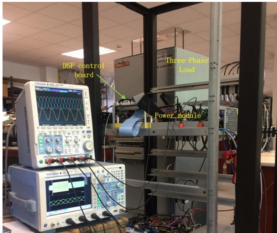
Fig. 6. The prototype of the NPC three-phase three-level topology based UPS platform.
