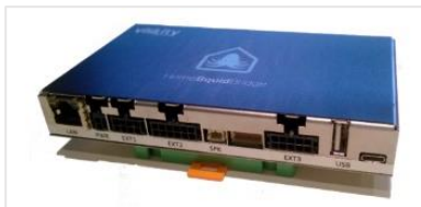
Figure 4-6 Gateway of the window system (Visility ApS).
