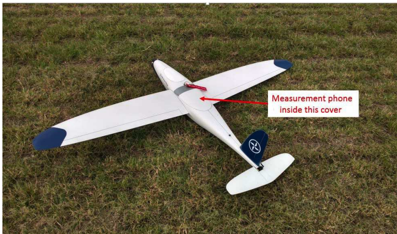
Fig. A.1: Cumulus One. UAV used for measurements
