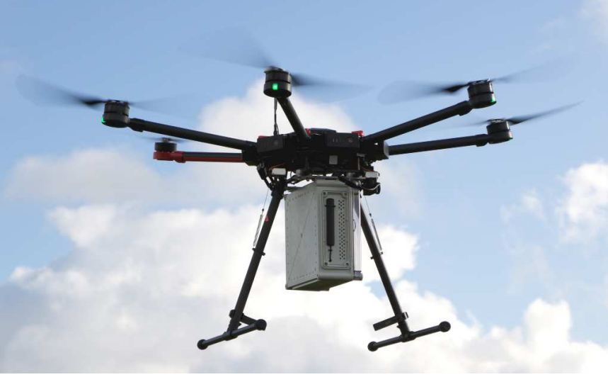
Fig. F.1: The measurement equipment mounted on the drone is monitoring live LTE networks.
