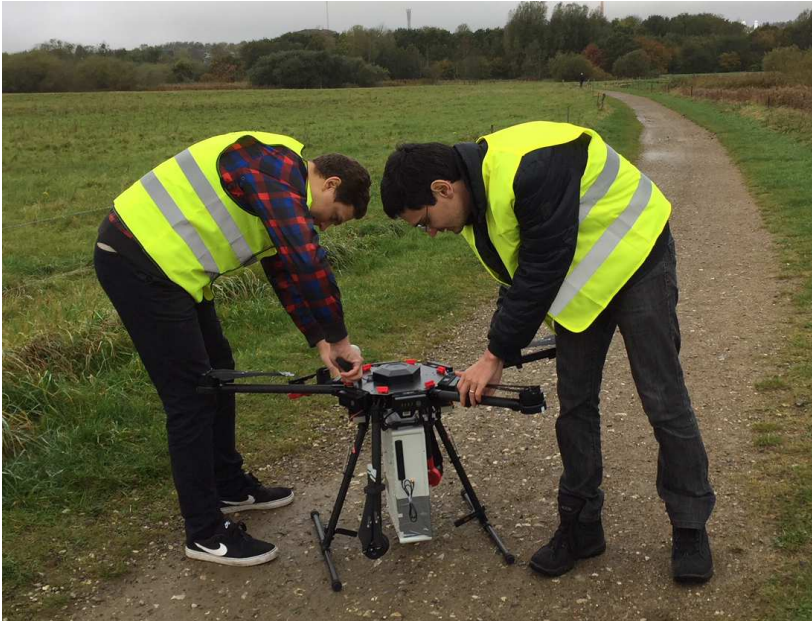
Fig. G.1: Preparation for UAV channel measurement: Our pilot is mounting the R&S scanner on the DJI Matrice 600 drone.
