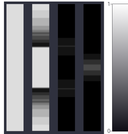
Figure 3. Textures used for the marimba bar, with intensified brightness. The grayscale value of the color is the modal weight. The leftmost depicts the fundamental frequency while the rightmost in the connected field depicts the fourth mode. In this instance, all other position’s weighting values are scaled compared to the fundamental frequency, the modal texture of the fundamental frequency is a single value across all positions.
