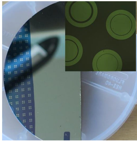
Fig. 1. Photo of a half-wafer with ring-shaped contacts (left) and continuous films (right). Insert represents 10x-magnified optical microscope image showing the contact structures.
