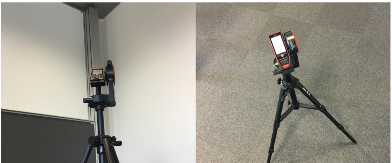
Figure 2.2 Using the handheld laser with a tripod
