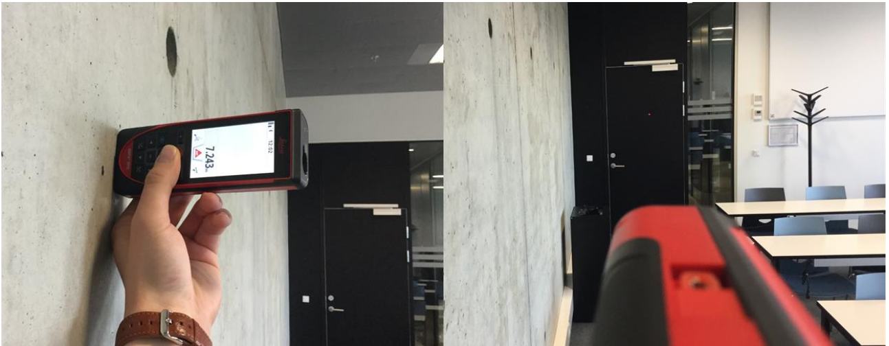
Figure 2.1 Using the handheld laser as an advanced measuring tape by placing it in on a surface and measuring the distance to the surface opposite the placement surface.
