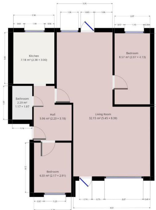
Figure 5.6 The test case floor plan modelled in Magicplan.
