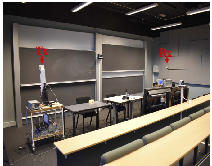
Fig. 12. Short-range indoor measurement with a Tx-Rx separation distance of 5.8 m.
