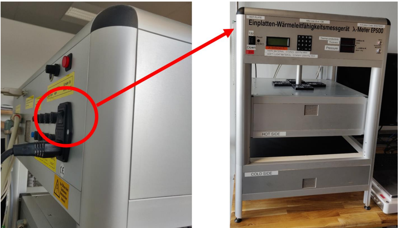
Figure 18: Power switch button on the rear panel of the Guarded Hot Plate Apparatus (left). Location of the power switch button seen from the front of the Guarded Hot Plate Apparatus (right).
