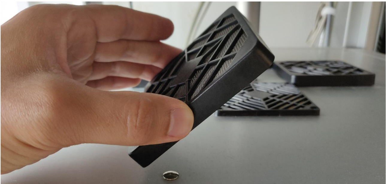
Figure 7: Dismounting the plastic cover of the ventilation filters.
