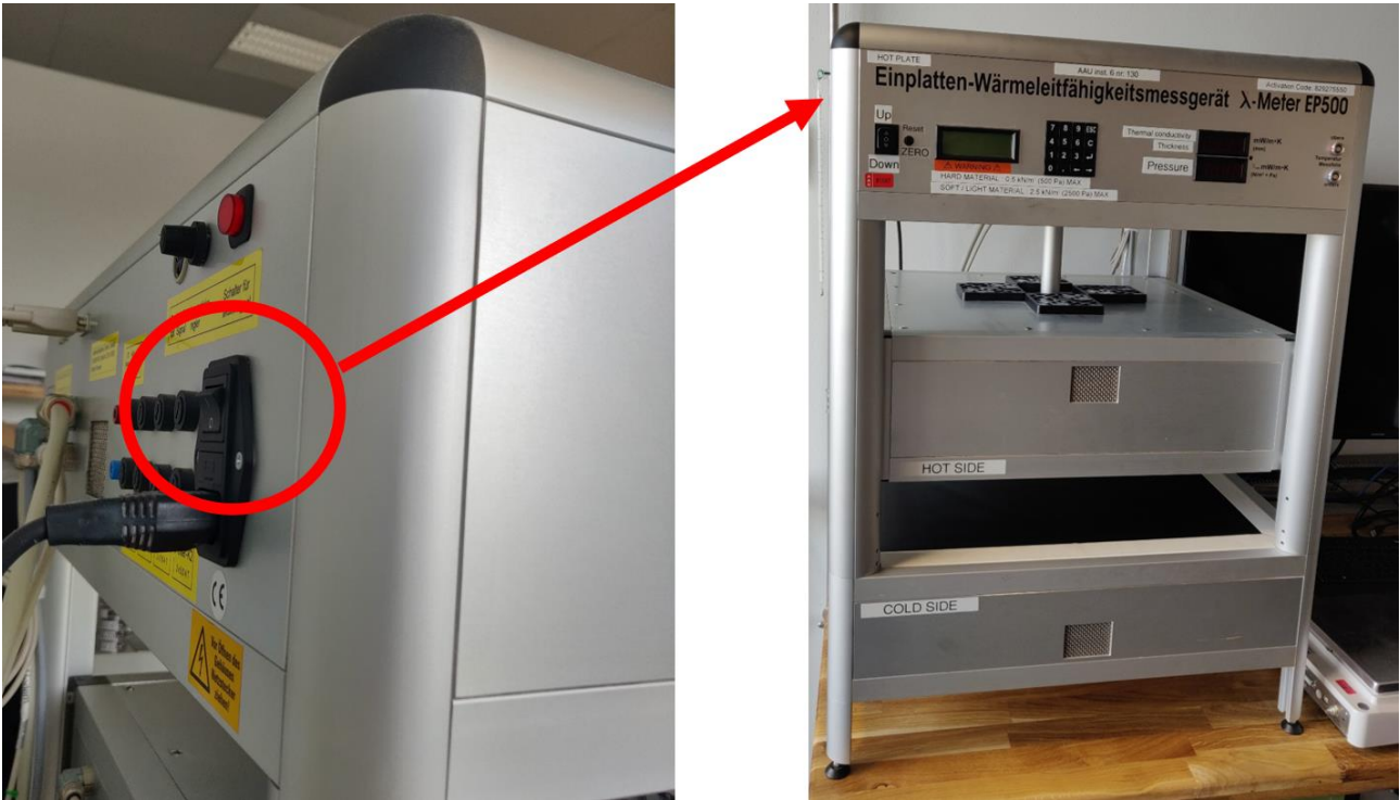
Figure 3: Power switch button on the rear panel of the Guarded Hot Plate Apparatus (left). Location of the power switch button seen from the front of the Guarded Hot Plate Apparatus (right).
