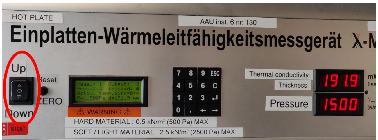
Figure 16: Press the "up" button to open the middle component of the apparatus.
