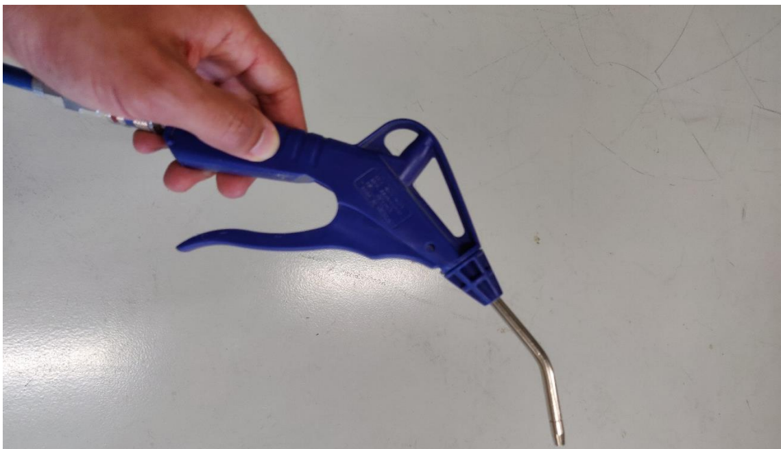
Figure 9: Pressurized air to clean up filter pads.
