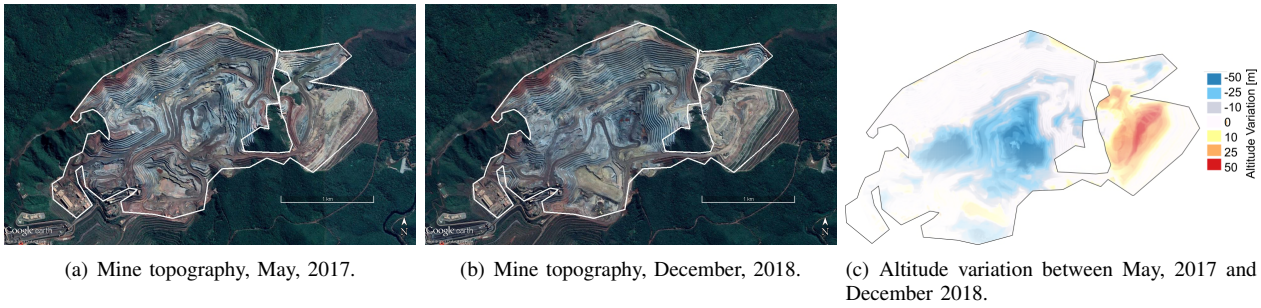
Fig. 1: Mine topographic variation between both measurement campaigns. The area of interest spans 3 by 4 km
