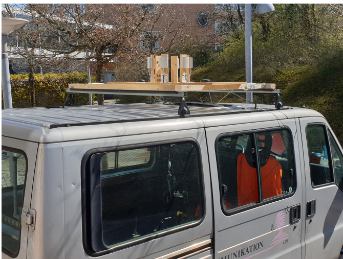
Fig. 2: A measurement vehicle with the antenna structure on the roof
