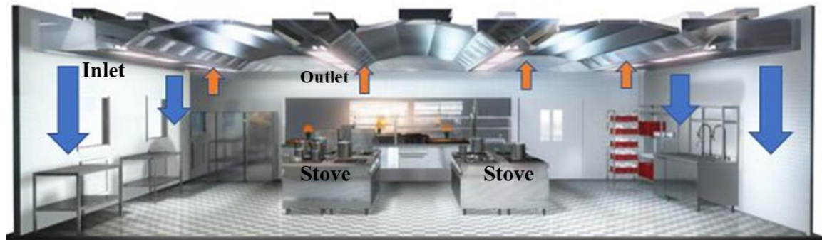
Fig. 31. Ventilated ceiling with air curtain ventilation.
