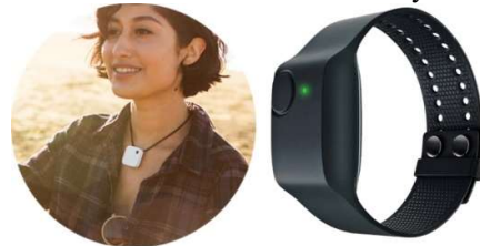
Fig. 2. Left - Narrative clip lifelogging camera, Right - Empatica E4 wristband.
