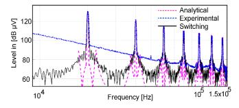
Fig. 8. Obtained eperimental and analytical and switching model for EMI peak measurement (Band A) with switching frequency (fsw = 20 kHz).
