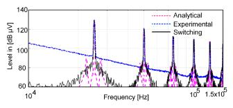
Fig. 10. Obtained eperimental, analytical and switching model for EMI peak measurement (Band A) with switching frequency of fsw = 25 kHz.
