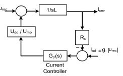
Fig. 5. High-frequency dynamics block diagram of single-phase boost PFC converter adopted from [16].
