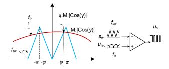
Fig. 3. The voltage across the switch  $(u_s)$  in CCM mode operation in a boost PFC converter.
