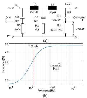
Fig. 6. a) Circuit of LISN in band A according to CISPR 16 b) Impedance frequency behavior of LISN.
