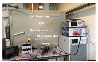
Fig. 7. Photograph of the test setup for Boost PFC converter.
