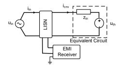
Fig. 4. Thevenin equivalent circuit of the simplified boost PFC converter.
