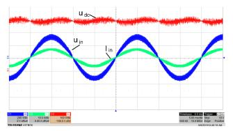
Fig. 9. Measured experimental waveform of a single phase PFC rectifier with following Table1( $f_{sw}$  = 25 kHz).
