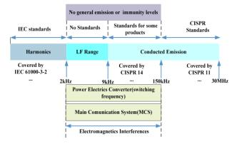
Fig. 1. Harmonic and conducted EMI frequency range classified by IEC for electrical network [6].
