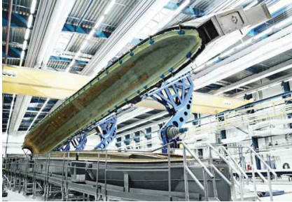
(c) The upwind and downwind parts have been infused with resin and are now about to be glued together.
