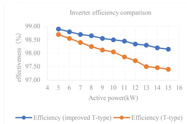
Fig.13 Efficiency comparison between improved T-type three-level inverter and T-type three-level inverter
