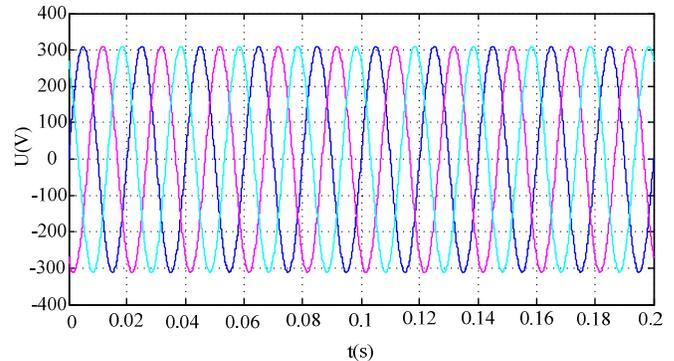
Fig.10 the three-phase output voltage of the inverter
