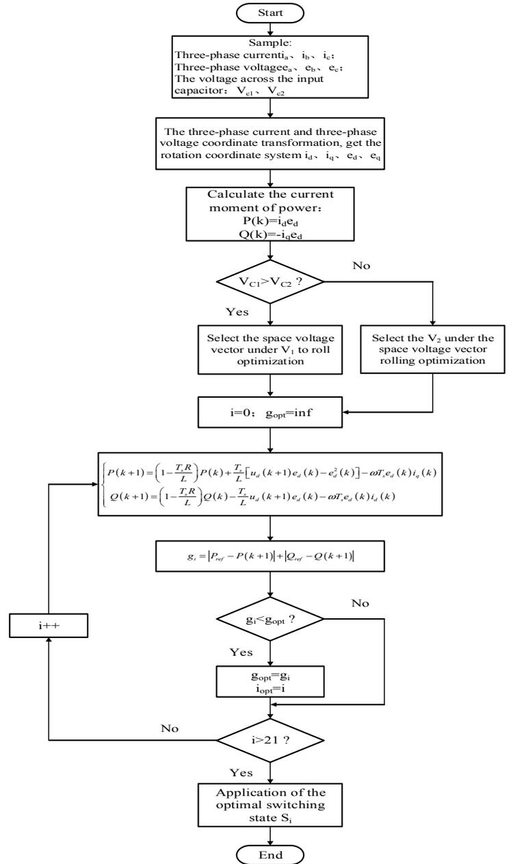
Fig.7 The model predictive direct power control scheme of improved T-type three-level inverter
