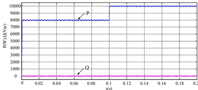
Fig.12 The active and reactive power waveform
