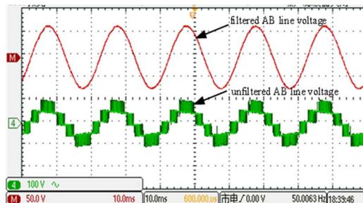
Fig.17 The output AB line voltage experimental waveform
