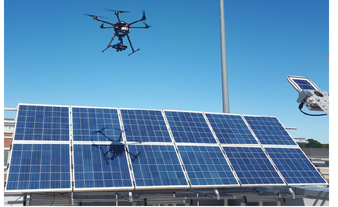
Fig. 7. Aerial drone based EL measurements shading the panel while performing outdoor measurements when camera is approximately perpendicular to the imaging panel.
