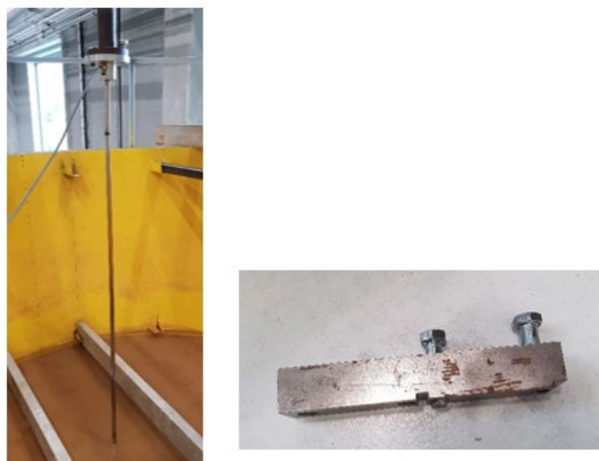
Fig. 3.9. The attached CPT device and the extension arm for the CPT.
