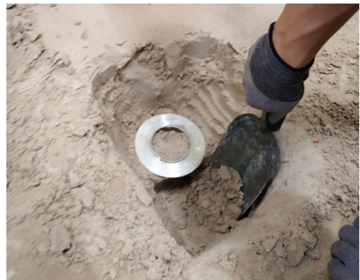
Fig. 4.13. Taking out the sample for D_R direct measurement
