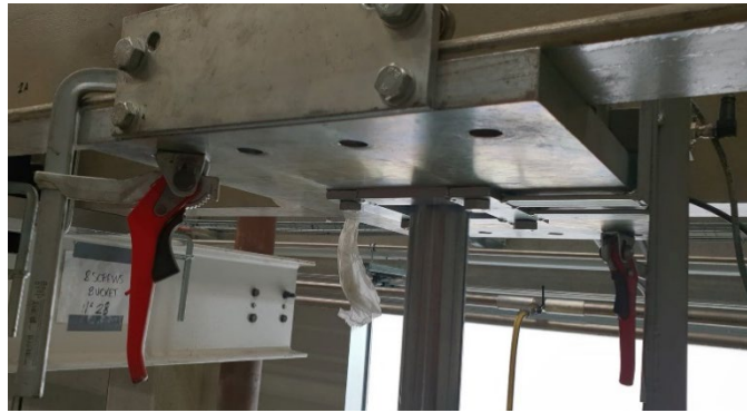
Fig. 4.2. The piston clamped with two clamps in opposite corners
