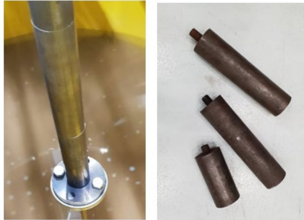
Fig. 3.5. The extension pieces for the piston
