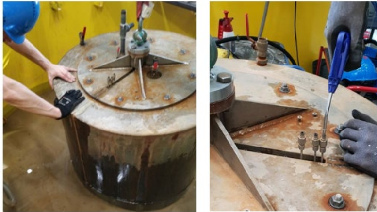
Fig. 4.11. Holding the bucket when lifting it; cleaning the bucket outlets with air piston
