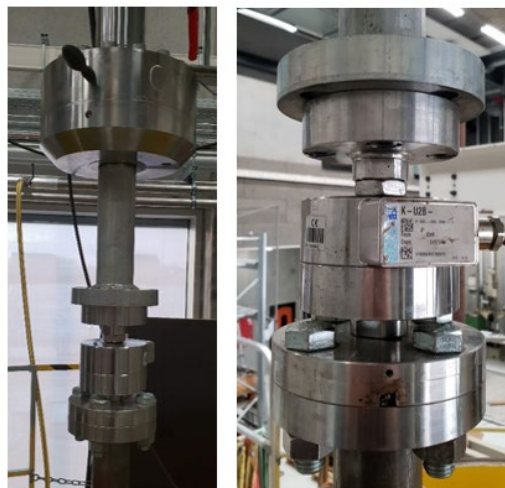
Fig. 3.6. Both load cells on the piston (left picture) and the connections on the small load cell (right picture)
