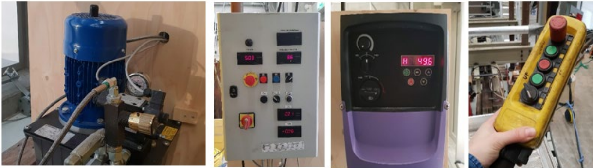
Fig. 3.4. Hydraulic system: hydraulic pump, control switchboard, setting switchboard and manual pilot for control (from the left side respectively).
