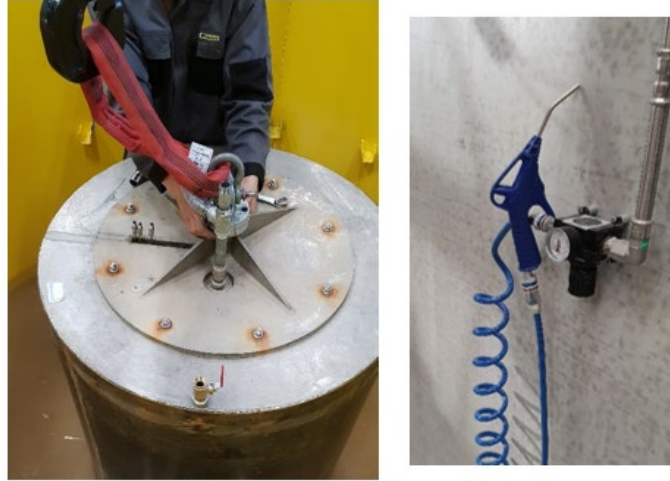
Fig. 3.10. The connection of the bucket model on the crane; the air piston
