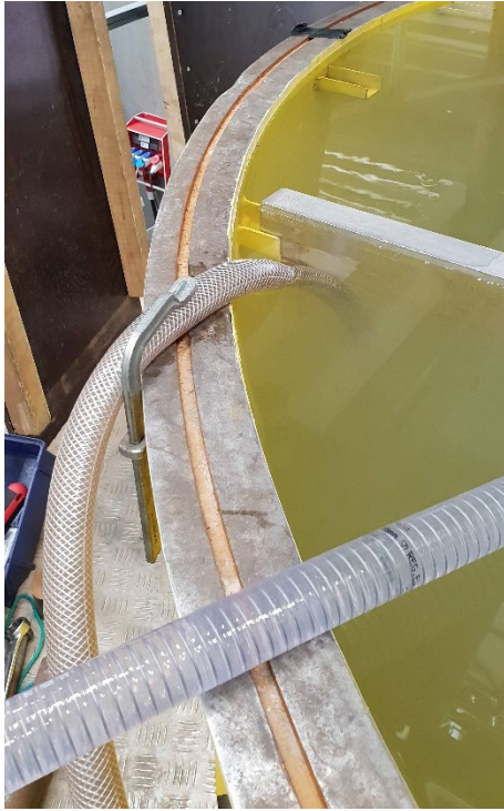
Fig. 4.9. Clamped outlet hose from suction pump
