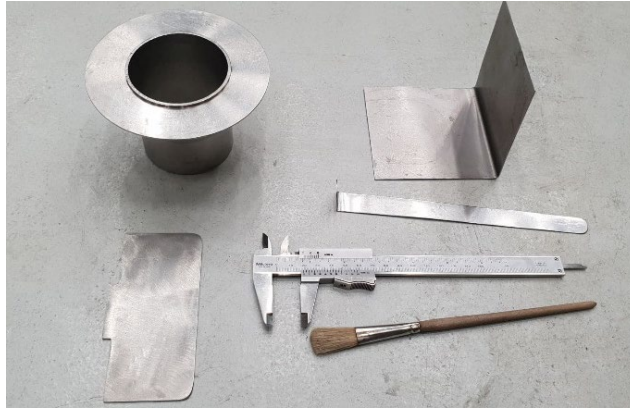
Fig. 4.12. Tools for the unit soil weight test: cylindrical molder, cutting tool, levelling tool, the hook for removing some sand from the molder, measurement tool and brush.
