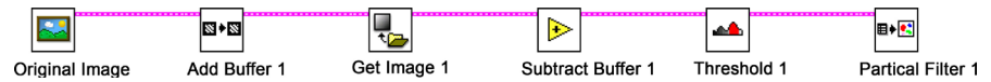
Figure 3. Image processing steps in NI Vision for detection of the textile inside the volute.
