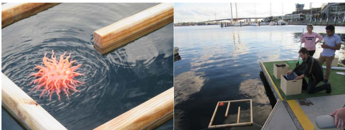
Figure 8: The water robot in its custom-built course. To the right, a young man is controlling the water robot through a floating box with a tablet controller inside, which he cannot see (Source: Authors).
