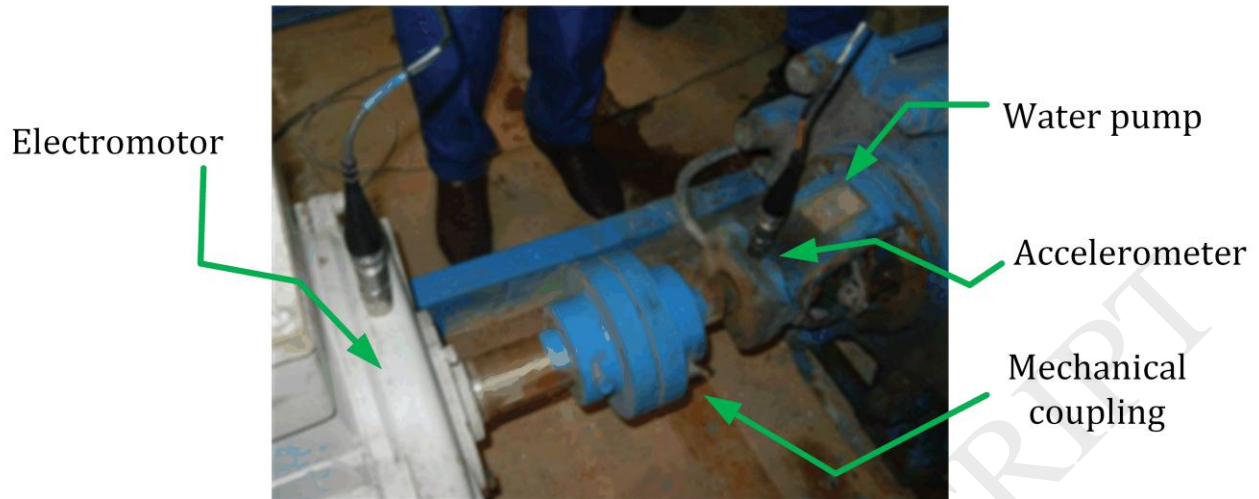
Fig. 7. The water pump connected to the accelerometer
