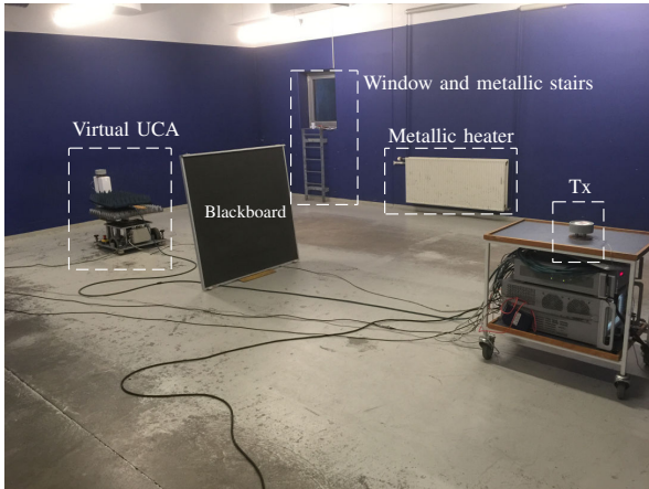
Fig. 2: The basement where the measurement campaign was conducted. (a) The top-view sketch of the basement. (b) A photo taken during the OLoS measurement.
