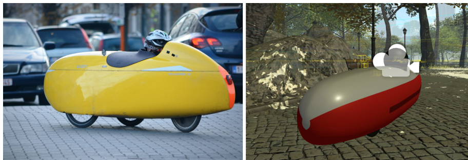
Fig. 2. Left: A cabin-based recumbent bike. Right: A 3D model of the bike in Unity5.
