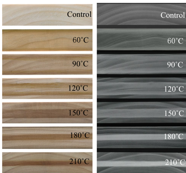
Fig. 1 Photograph images (left) and soft X-ray images (right) of transverse section of sandwich compressed wood preheated at different temperatures
