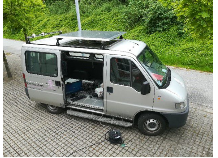
Fig. 2. A van with measurement equipment (inside) and antenna array mounted on a ground plane (roof)
