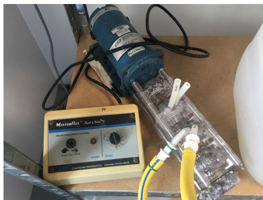
Figure 2 Masterflex peristaltic tubing pump
