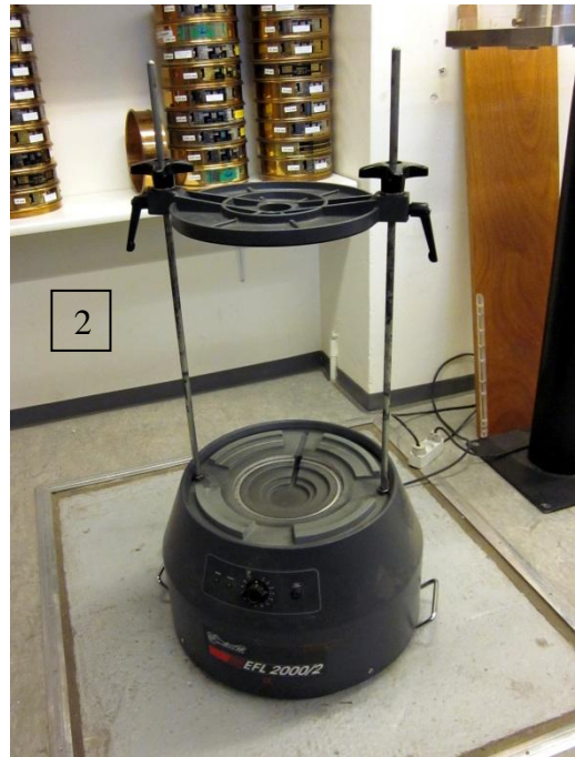
Figure 1: Sieves used for coarse and fine screening, and a shaker machine
