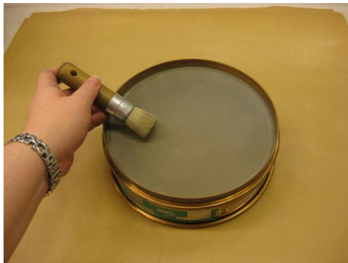
Figure 7: In order to empty the sieves, light brushing can be done on the backside of the sieve when placed on a large piece of paper.
