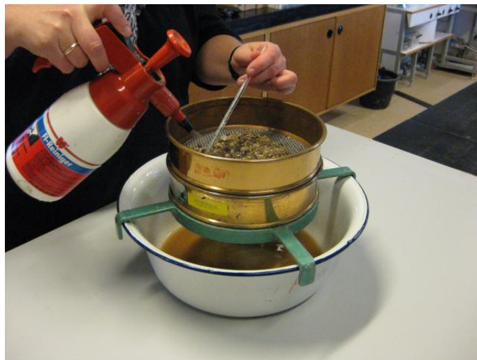
Figure 4: Wash out on 2 mm and 0.063 mm sieves.
