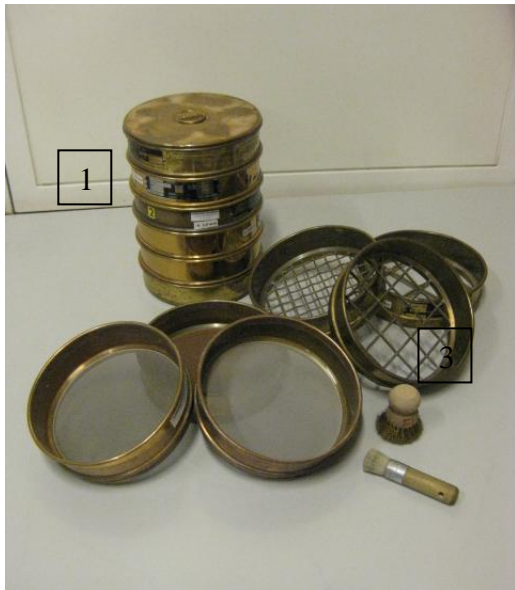
Figure 1: Sieves used for coarse and fine screening, and a shaker machine
