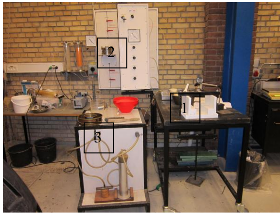
Figure 1: Simple failure apparatus with control panel plus special vacuum cleaner.
