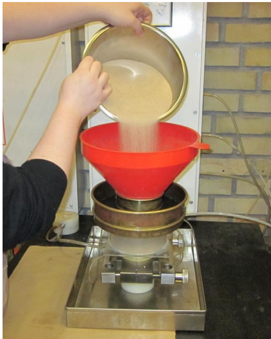
Figure 11: Embedding of sample.
