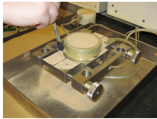
Figure 13: Levelling the sample and cleaning the membrane.
