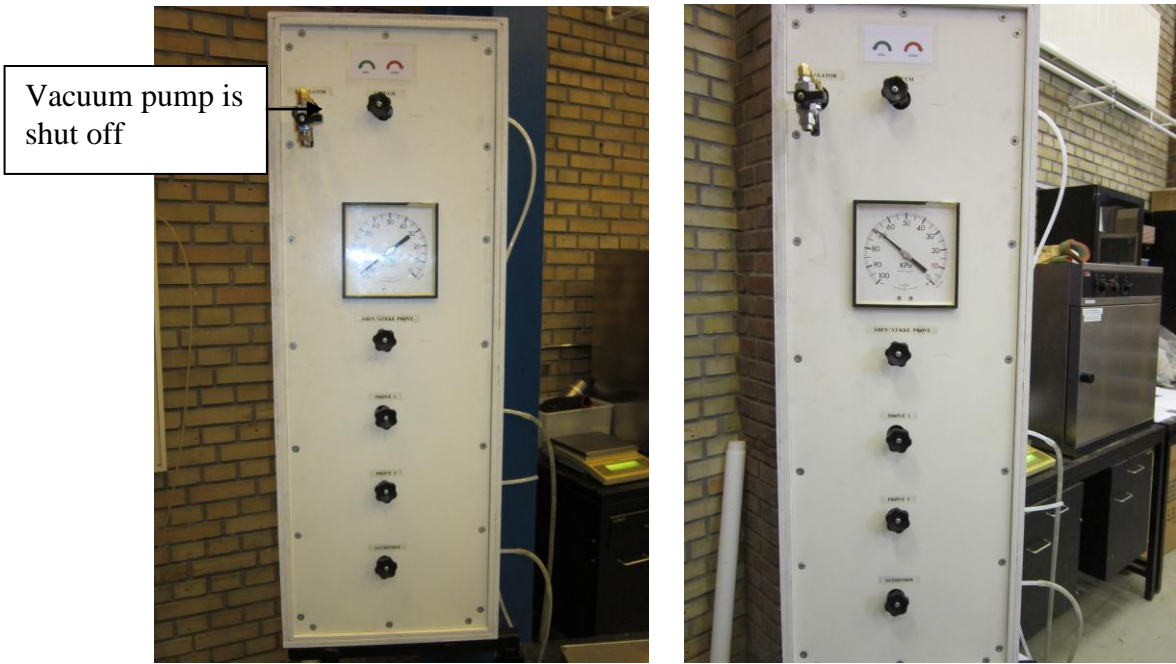
Figure 19: Vacuum pump is shut off on the control panel during the experiment.
