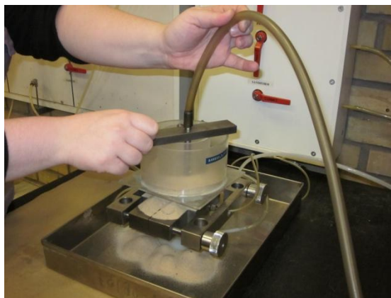
Figure 12: Vacuuming excess material.
