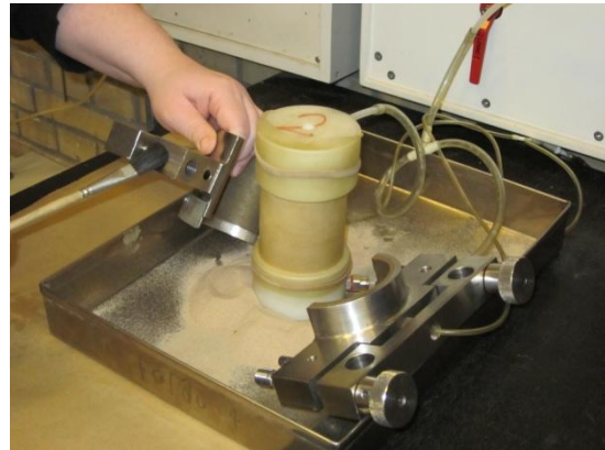
Figure 16: Sand mould is removed and sample is brushed clean.
