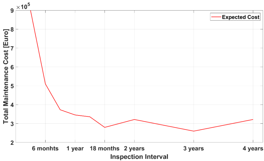
Figure 21 Cost Trend as Function of Inspection Interval for the Case of Almost Linear Damage Propagation – Decision Alternative 4
