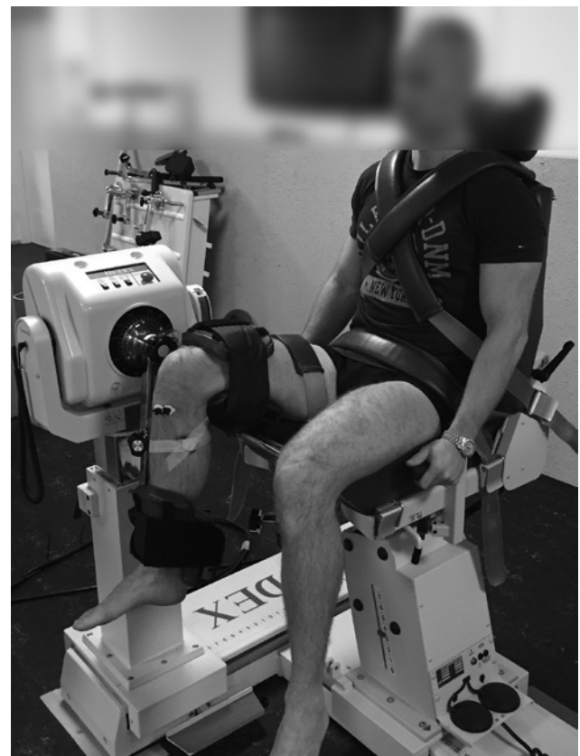
Fig. 1: The picture illustrates the experimental set-up using the isokinetic dynamometer. Here, the participant was comfortably seated with the trunk and lower extremities securely fastened with straps. The lever arm of the biodex passively moved the leg towards extension at a speed of 5^\circ/\text{s} . The participant was instructed to press a button when the stretch sensation in the posterior thigh changed to pain.
