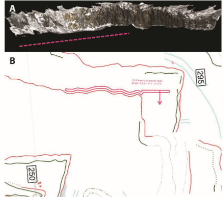
FIG 4 – (A) Mine block wall (220 m long) in Leveäniemi pit, located immediately west of the experimental transect that is shown as a dashed line. Note the conspicuous occurrences of fault lines and shear zones (see geological description). White areas are snow and ice; photograph November 2016, courtesy of mine geologist Celine Debras. (B) Location of experimental transect (140 m long) on level 280 in north-eastern part of Leveäniemi open pit mine. Arrow is indicating blast direction of experimental transect towards the middle/lower part of the pit.
