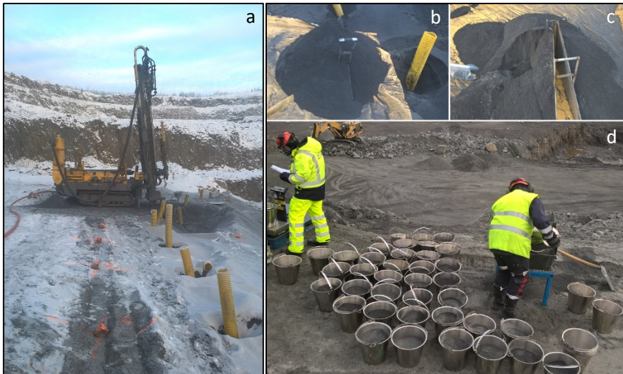
Figure 27. a) RC drilling during variographic experiment (paper III), b) sectorial sampling frame in BH cone (paper II), c) extracted manual BH sample and segment BH sample during variographic experiment (paper II), d) weighing and sample division during full cone BH reference sampling (paper II).
