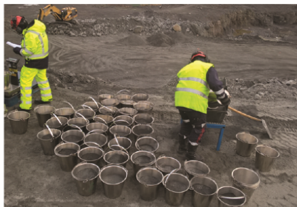
FIG 8 – Complete coarse cone and fines cone were collected in buckets, weighed and split in the field.
