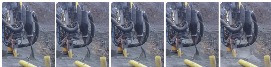
FIG 13 – Variability in the flux of blasthole coarse discharge from the D65 drill rig during experimental drilling.
