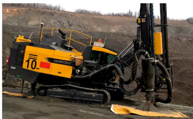
Figure 2. Experimental drilling with a canvas located under the fines cone discharge (rear end) and a canvas and sectorial sample frame located under the coarse cone discharge under the front discharge cyclone of the Atlas Copco D65 drill rig.
