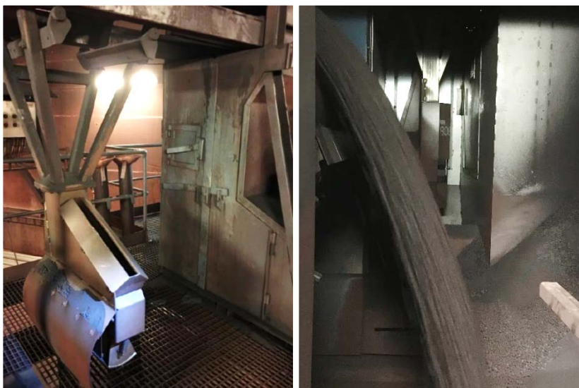
Figure 8. Two examples of linear cross stream samplers used in the pelletizing plants and Narvik harbour respectively. Left: Linear sampling bucket in maintenance position outside the ore stream. Right: Linear sampling bucket in rest position behind the belt discharge. (Photo: Jonas Gunnare)
