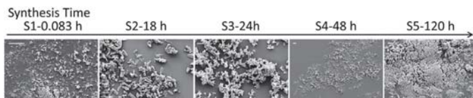
Fig. 2. SEM micrographs of S1–S5 from left to right. Each scale bar corresponds to 10 \mu\text{m} .
