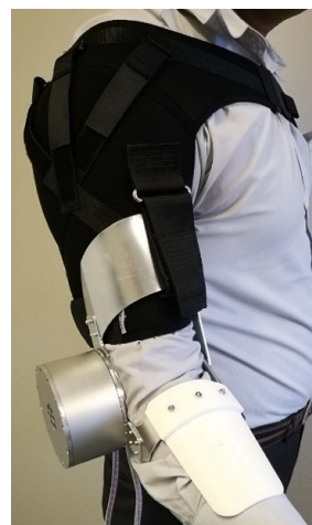
Figure: Version 2.1 of the integrated joint unit and elbow exoskeleton prototype
