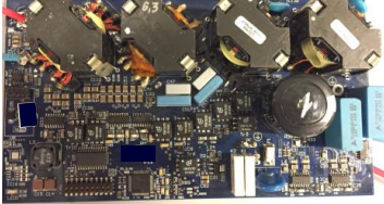
Fig. 2. Photo of the built PV microinverter prototype.
