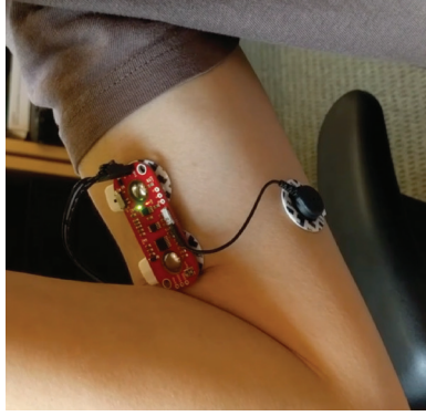
Figure 1: The MyoWare Sensor mounted on the bicep in the appropriate location according to [1].
