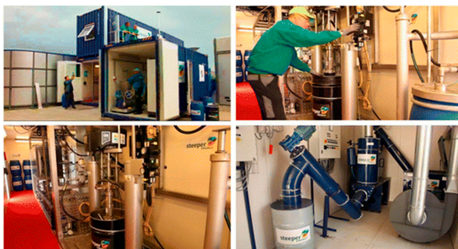
Figure 6. Operations of the Hydrofaction™ process at the pilot plant at Aalborg University, operated by Steeper Energy. Reproduced from [13], with permission from Springer, © Springer-Verlag 2017.
