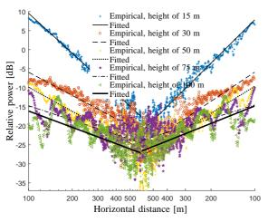
Fig. 15: Power fittings for the five horizontal flights.
