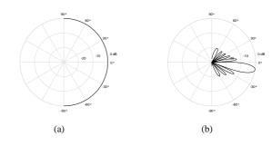
Fig. 11: Generated BS antenna radiation patterns embedded in the GM. Note that the backwards patterns are not illustrated. (a) Omnidirectional elevation pattern. (b) Directive elevation pattern with half power beamwidth of 10° and downtilt of 10°.
