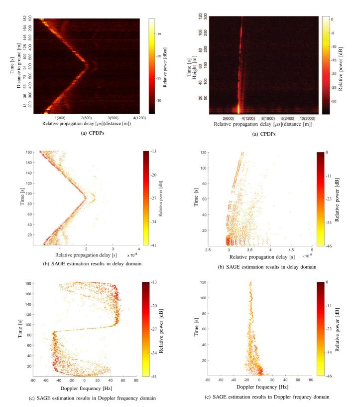
Fig. 7: CPDPs of a horizontal round-trip flight at the height of 75 meters and corresponding SAGE estimation results.
