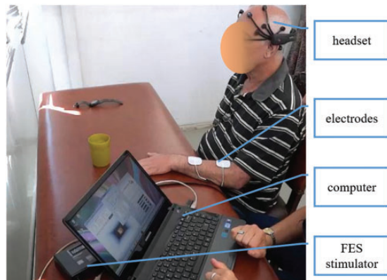
Figure 4. A patient using the Emotiv_BCI-FES System . The different elements of the system are visible in the picture: the headset for EEG signal acquisition; the computer where the software for the BCI and the interface run; the FES device and the electrical stimulation electrodes placed on the extensors of the wrist.
